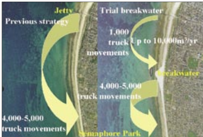
Figure 4.6 Distances and number of truck movements for sand to be carted to Semaphore Park from (a) south of the Semaphore jetty (previous strategy) (b) the Semaphore jetty and south of the Semaphore South breakwater (Semaphore Park Coast Protection Strategy)
